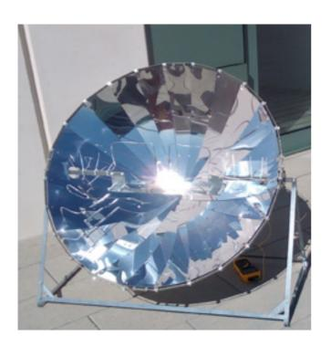
The Nanoengineering of Materials Applied to Energy (NEMEN UPC) group has developed a photocatalyst that can produce hydrogen with solar light from contaminated water. The photocatalyst, which contains a titanium oxide semiconductor and small clusters of metals, has been developed through the Single-Atom Catalysts for Hydrogen Photogeneration (CMIRA) cooperation project, together with IRCELYON.
