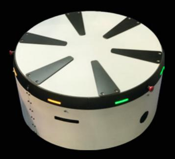
The Industrial Equipment Design Centre (CDEI UPC) has developed a new system for omnidirectional movement that can move forwards, backwards, sideways and diagonally, with independent rotation and great accuracy. One of its main advantages is that it reduces the space needed to perform the desired trajectory, increases the ability to adapt to different environments and facilitates interaction with different machines.
